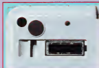
The CD-ROM will connect to the Super Nintendo through the port on the bottom of the Super NES.
